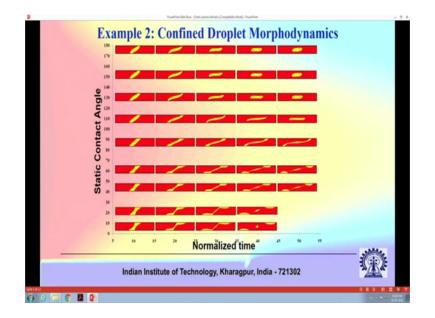
In the next example I will talk about confined droplet dynamics. This is a very interesting area and in micro fluidics droplets are studied for many reasons, I will not get into the details of this slide, but the whole idea is to let you know that how a droplet morphologically evolves based on the wettability of the surface on which it is there. So, that diagram is shown in this slide this is entirely a computational exercise.
