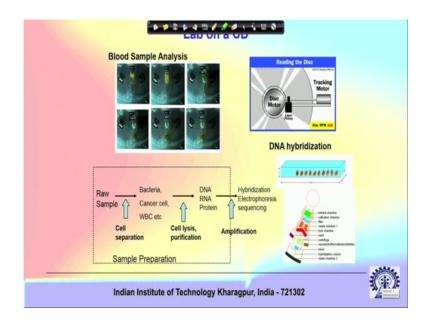
The next concept that I talk about is lab on a CD; which briefly we have touched upon earlier. So, in a lab on a CD the advantage is that in the paper based device to do a large number of tests you need to make a large number of channels on the paper. And there may be a limitation of fabrication and other things so that is itself an important design job.
