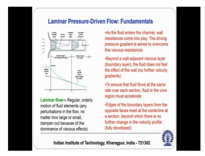
So, you see here that the fluid enters the pipe with a velocity profile such that there is a layer close to the solid boundary where the viscous effects are important, but as you go away from the solid boundary the viscous effects become less and less. So, this layer
