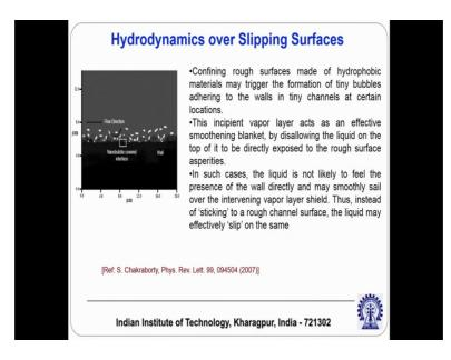
So, that is one of the very important considerations and there has been lot of research work actually in this domain to understand hydrodynamics over slipping surfaces. So, it is important because if you try to understand how you can control the slipping of fluid over a very rough surface, rough and hydrophobic surface can promote slip in a confinement research has shown this.
