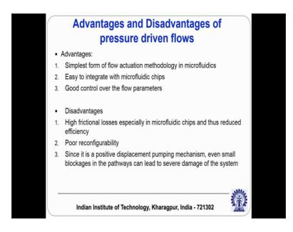
So, we will summarize the discussion or conclude the discussion in this lecture by pointing out advantages and disadvantages of pressure driven flow. So, for that I will refer to the slide, the advantage of pressure driven flow is that it is the simplest flow actuation right you we just need a need a syringe pump to drive the flow.
