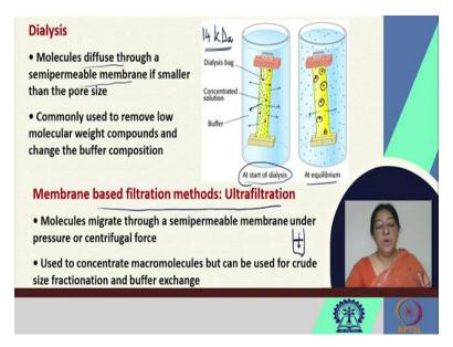
Now that we have our protein present in our fraction, we want to get the protein from the concentrated solution. So we have the molecules diffused through a semi permeable membrane in a process called dialysis, where it is commonly used to remove low molecular weight
