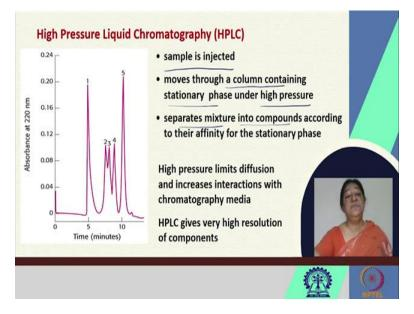
As we do so, we can look at a method called high pressure liquid chromatography. Here we have the movement through the phase under high pressure. This separates the mixture into the compounds according to their affinity for the stationary phase. This is a method that limits any diffusion possibilities because of the high pressure being applied and it gives very high resolution of our components.
