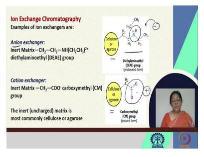
In ion exchange chromatography, we look at anion exchange, where we have the protonated form of the gel matrix. This being positively charged, any negatively charged protein will get attached to it. So this is an anion exchanger. Similarly, we can have a cation exchanger, where our resin is negatively charged and our protein that would bind to this is positively charged.
