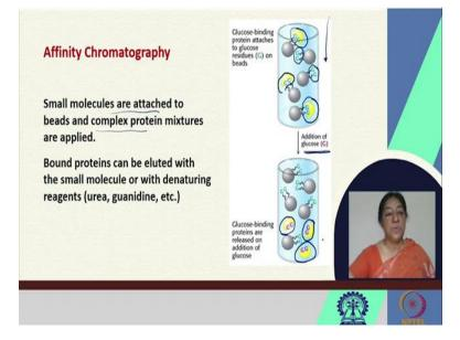
We have affinity chromatography where we have for example, a protein that has an affinity for glucose. In this case the protein binds to the glucose. The yellow protein that we see here [refer to slide] binds to the glucose and the small molecules are attached to the beads and the mixture of proteins is in the column. Now anything that has an affinity for glucose binds to the beads.
