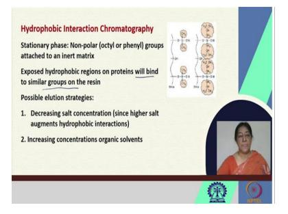
We can also have a separation based upon the hydrophobic capacity of proteins. In this case exposed hydrophobic regions of the proteins will bind to similar groups on the resin. Then how do we remove this?
