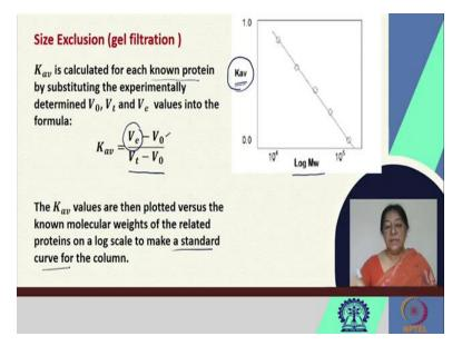
$K_{av}$  is calculated for each known protein, we have a set of known proteins for which the molecular weights are known. Here we have the log molecular weight and the  $K_{av}$  value, depending upon the column used and the conditions for the illusion the experiment is conducted, where we have the  $V_t$  -  $V_0$  corresponding to the column.
