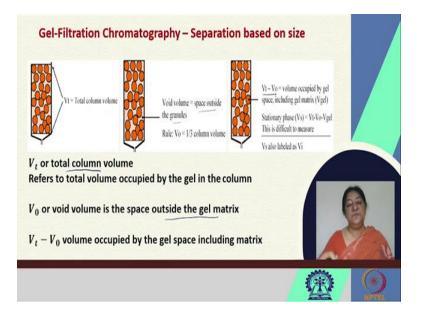
There are certain terminologies that we need to know here. There is a total column volume that is the total volume that is occupied by the gel in the column. We have the void volume that is the space outside the gel matrix or outside the granules, which needs to be also known to determine the partition coefficient. This means that, the volume occupied by the gel space including the matrix is  $V - (V_t - V_0)$ .
