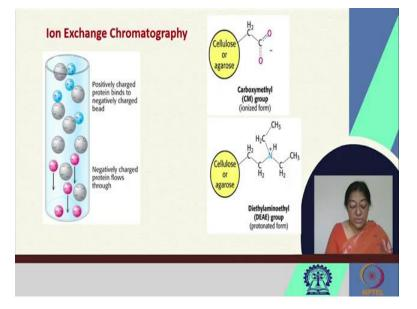
If we have negatively charged beads as is seen in this case, any protein that is negatively charged would not bind to the column but would appear as it is called in the flow through.
