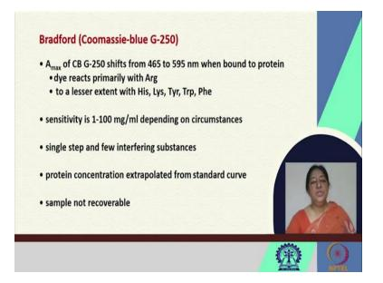
Another method is using a dye, where the absorption maximum shifts from 465 to 595, when this coomassie-blue G-250 is bound to the protein because it reacts primarily with arginine and we have a good sensitivity. So we can take a drop of our eluted sample and mix it with the Bradford reagent to see whether we have our protein of interest.
