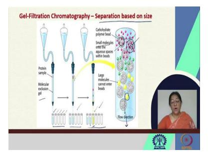
In gel filtration chromatography we have separation based on size. This is also called size exclusion chromatography or molecular sieve chromatography. In this case what happens, we have a carbon polymer bead which has within it a network. In this network the smaller molecules can enter the network; the medium size molecules will partially enter the network, while the larger molecules cannot enter the beads and are removed first.
