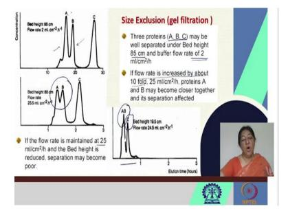
If we look at certain methods or certain important parameters, we have a bed height of our column and we have a flow rate. We want to separate out three proteins based on size exclusion with different molecular weights. Ideally we would want the A, B, and C to form distinctly different peaks.
