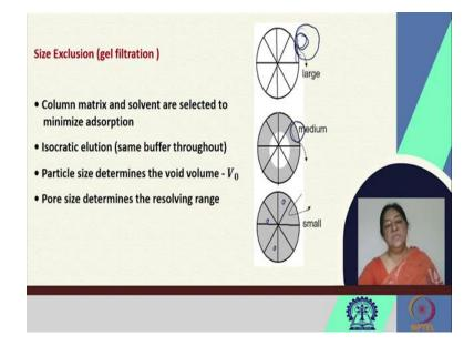
In this size exclusion or gel filtration chromatography, we realize that the larger molecule will not be able to enter the bead, a medium size molecule may partially enter the bead, but a smaller size molecule will definitely enter the bead.
