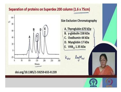
In a typical size exclusion chromatography, chromatogram as it is called, if this [refer to slide] is the column dimensions, we have 5 proteins here. We see in the minutes that have been elapsed through the column running, we have molecule A come out first followed by B C D and E. So A comes out first and D comes out last, indicating that A has a large molecular weight and E has the smallest molecular weight.
