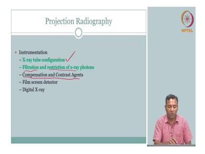
So, in the instrumentation, we started with the X-rays right, the X-ray tube configuration and then, just after the x-rays come out of the x-ray tube which is going to be a spectra of energy, we wanted to do two things; one is do the filtration so that only the energies that have maximum probability to give you signal right.
