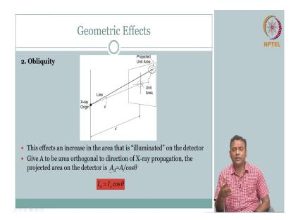
Next is your geometric effect is a obliquity. As a what is oblique? As you can see here in the I have a detector we were talking about detector being perpendicular so that the source is coming and hitting and the object plane and your detector plane are parallel to each other right that is what we were drawing in. But, what if there is some angle right if it is not perfect some angle that is called as your obliquity, but when we talk about some angle, where is its effect?
