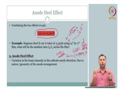
So, one of that effect that is more dominant is actually the Anode Heel Effect. What does this anode heel effect represent? Again, this is also due to geometry. Why is it grouped under geometry? Because, there is something to do with the setup geometry of the set up. But then, unlike the other two where it was the source to distance, source to object distance or the source to detector distance of that geometry.
