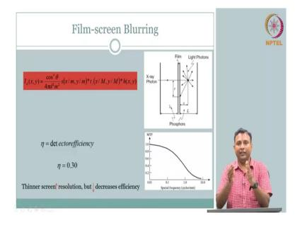
So, here, the only aspect that is there on the detector is your film screen, otherwise there is no big deal. So, we covered film screen. So, in the film screen what we talked about is you add a X-ray film and on both sides you add phosphor. Remember the cascade packing. So, you get the X-ray photon, X-ray photon comes, it generates light photon. So, here you have a one
