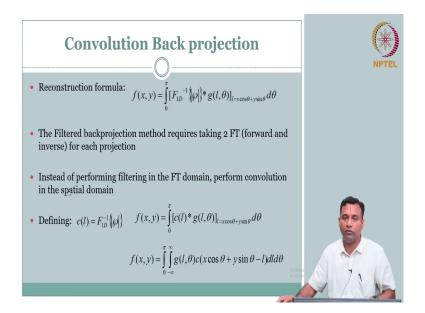
I like filtered back projection, but you know what why should I do the filtering in frequency domain; why cannot I do in time or space domain? You can quickly recognize ok what is frequency domain, you multiplied; if you have to apply the filter in spatial domain, it has to have convolution, convolution back projection. So, it is I mean small way it is a it is a variant and the reason for that is, it is convenient to operate, ok.
