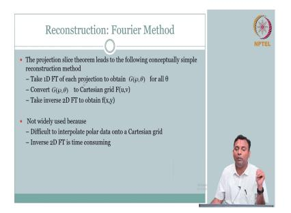
So, now get back to all the reconstruction, from now on it is a breeze; we are going to cover beautiful algorithms right, but you know a big picture, that is all it is straightforward, ok. So, first is Fourier method, what do we mean by Fourier method? Directly from the projection slice theorem, we know what to do; what we have got is, we got one projection, take the 1 D Fourier transform of it, right.
