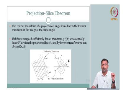
So, the Fourier transform of a projection at an angle theta, Fourier transform of a projection at an angle theta is a line in the 2 D Fourier transform of the object at this along the along the origin at the same angle. So, if I did a projection at 0 degree, then in the Fourier domain that 1 D Fourier transform of the projection will sit along the 0 degree line or same angle of your u comma v space.
