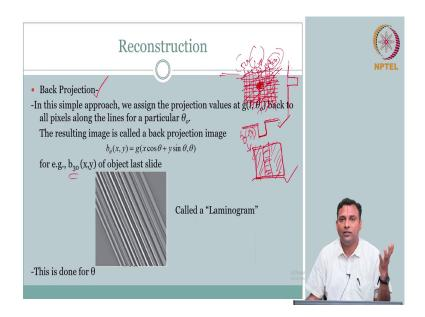
So this is for one angle, this image is called as a Laminogram ok; because you can see laminates line feature, so this is Laminogram. So, what can you do? This is just one example, we can do this for all the theta, right. So, you can in fact reconstruct this b right at all the different thetas as well, which will be very similar to this. So, you get several different Laminograms.
