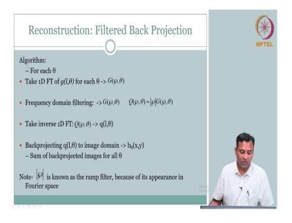
So, what you have done just to recap? For each theta you have taken the Fourier transform of for the projection, right. So, you have g of l comma theta is measured at different. So, the projections are measured for different theta. So, for each theta you take the 1 D Fourier transform, you get G of capital G right your frequency domain representation of your capital G.
