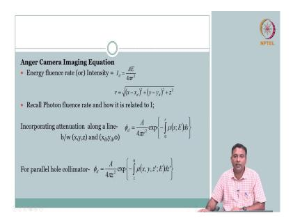
So, if you have the anger camera the equation you can write the intensity as radio activity into so number of photons right into E energy per photon. So, this would be your intensity falling on the detector where r is just the distance from x y z to your location on the detector right x comma y comma x d comma y d comma zero ok.
