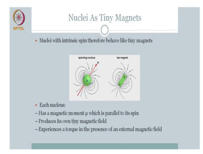
So, I said you could imagine that it is very similar to a bar magnet a bar magnet has a North Pole South Pole it has magnetic flux lines. So, it will align itself to the Earth's magnetic field like this you have your charged particles that is spinning. So, you have a magnetic moment vector mu.
