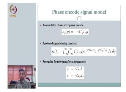
So, what is the signal phi y is the accumulated phase for the duration over which you are applying the phase encoding gamma G y T p and whenever it is at y. So, it is gradient is applied along y direction right G y y. So, this is the maximum phase will be G y T p y ok. So, your phase is given like this. So, how does your baseband signal change out? In baseband signal, same as before only thing x is varying with the t read out direction near y direction you have this phase information.
