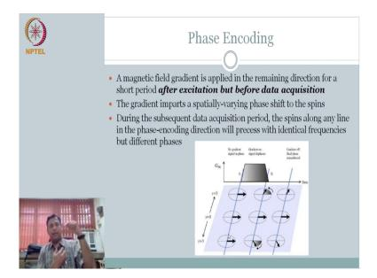
So, let us look at what phase encoding is. So, a magnetic field gradient again we exploited G e z we exploited G x which was called as G e z was called as slice selection; G x was called as readout or frequency encoding. Now you are exploiting the other direction G y, a magnetic field gradient is applied in the remaining direction in our case it is G y importance is when you are applying it.
