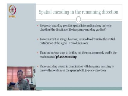
So, again so, the frequency encoding provides the frequency encoding when we talk about convention says, we are talking about x gradient. The frequency encoding provides spatial information only along the x direction, direction of frequency encoding. To reconstruct an
