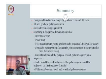
So, to summarize the data acquisition we covered design functions magnets, gradient coils all those things. We also covered the gradients pulse sequences and then we talked about slice selection is usually z gradient and then the forms of scanning rectilinear and polar scanning ok. We also made distinction between your T 2 start which is your dephasing due to change in magnetic field. And spin echo; that is due to your spin interaction that will come in your spin echo machine.
