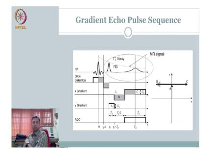
So, we can combined right you are combined your gradient echo and your phase encoding we can travel to the negative axis and move up and down in the u. So, this is the pulse sequence RF excitation, slice selection, refocusing. I am not recording the data. So, ADC is not your free induction decay here rather I am applying a phase encoding just after that, I am doing a frequency encoding and I am reading out the gradient echo during the frequency read out encoding right.
