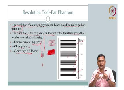
So, how do they do this, right; I mean this is fine, but how do they typically do, how do you calibrate, how do you say the imaging system resolution is one thing or the other? Most of the times, what they do is you have imaging system, you have a ground truth. So, the example that I showed here with a pen and a microphone, this is very arbitrary right, it is ok for a concept.
