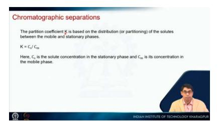
So, let us say we have a column and in that we have some gel matrix. So, the gel matrix will be the stationary phase, and the buffer or the solution in which your protein is dissolved is the mobile phase because it will pass through the column. So K is defined as  $C_s/C_m$  where  $C_s$  is the solute concentration in the stationary phase. So this s stands for the stationary phase, and  $C_m$  is the concentration of the solute in the mobile phase. So this m stands for mobile phase.
