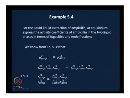
To get a little more comfortable with this, let us work out an example. For the liquid-liquid extraction of ampicillin, at equilibrium, express the ratio of the activity coefficients of ampicillin – that ratio is missing here – the ratio of activity coefficients of the ampicillin in the two liquid phases in terms of fugacities and mole fractions. Take about 15 minutes. Go ahead and do this please.
