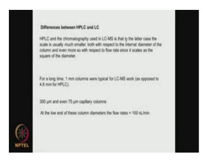
Now, what is the difference between HPLC and liquid chromatography HPLC and LC? LC is much smaller than HPLC and with respect to the internal diameter of the column and also with respect to the flow rate. Whereas HPLC may have higher flow rate and it may have larger diameter column. If you look at LC-MS, generally the column size
