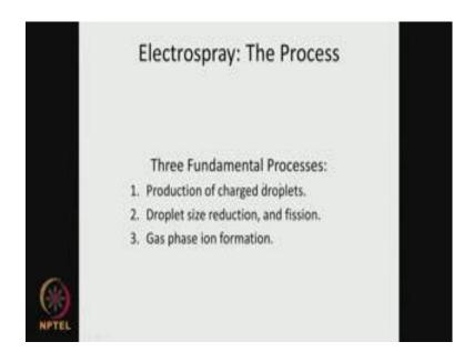
So, this process electro spray or ESI we produce charged droplets charged droplets droplet size reduction, so the droplet gets reduced, solvent gets evaporated gas phase ion formation. So, you have ions formed here, this is called gas phase because the solvent is completely evaporated during this process.
