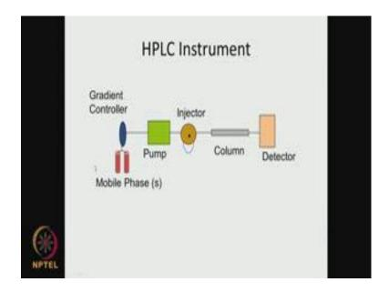
So, typically the HPLC instrument will look like this. We have a column, where we have a stationary phase we can inject the sample here the mobile phase could be one single solvent or it could be many solvents. And then it is pumped inside and it goes here to the detector after the separation. The detector could be your mass spectrometer, which I showed you before like this. This whole thing the detector could be mass spectrometer.
