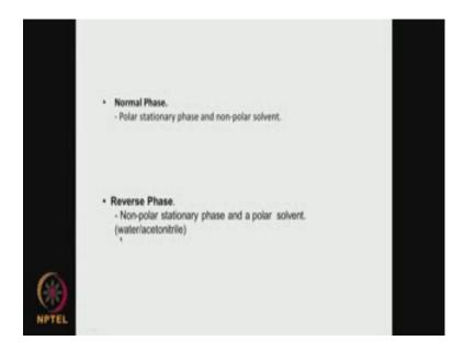
So, in HPLC or LC we have the normal phase that means, the normal phase is a polar stationary phase; and the solvent could be a non-polar solvent, whereas when you have a reverse phase the stationary phase could be non-polar or hydrophobic material, whereas the polar solvent could be water acetonitrile combinations of these and thereof actually. So, we can have a reverse phase liquid chromatograph, or we can have a normal phase liquid chromatograph.
