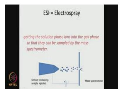
ESI is another technique; it is much milder, it is electro spray ionization. So, what we do is analyte and solvent together is injected through a small nozzle, we apply a very high voltage here. So, the particles or the stream coming out will be small diameter spray and it will be very highly charged. So, as it travels you can focus it and so these are the solvent gets evaporated, the analyte is now charged small particle, and it goes into your mass spec.
