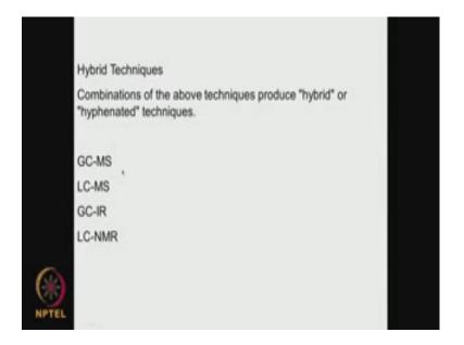
Now, let us look at each one of them little bit in more detail. So, we can have hybrid gas chromatograph mass spec, liquid chromatograph mass spec, gas chromatograph infra red, liquid chromatograph NMR. So, we can have many different types of these are called hybrid techniques hyphenated techniques. So, we can have the liquid chromatograph and the mass spec. So, both are possible.
