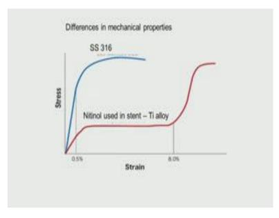
So, different metals have different types of stress strain diagram for example, stainless steel will look like this Nitinol is the titanium alloy it will look like this much lower and
