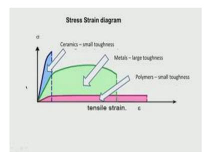
So, again same metals polymers ceramics. So, ceramics of course, do not have the plastic region they have only the very small elastic region modulus are very very high and as you can see polymers have the lowest modulus they are smallest toughness large toughness small toughness. So, this again this picture remember long time back we have been comparing polymers and ceramics in this fashion.
