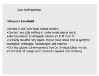
Because elevated chromium cobalt in blood and urine are observed in some cases they can even form non on a scale and large in number and like polymer other ions that are also released titanium aluminium vanadium nickel, but cobalt is the main chap that is a big problem in chromium cobalt toxicity can affect many organ organs neurological problem, cardiological problem, himatal hematological problem and endocrine problem.
