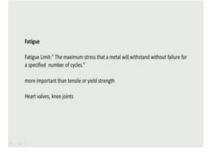
Fatigue is another important property which comes in of course, even in non metals the maximum stress that a metal will with stand without failure for a specified number of cycles for example, if you have heart valves it keeps on moving opening moving opening. So, that is how many times we can do that it is more important than tensile or yield strength because heart valves knee joints and all these undergo lot of fatigue. So, that is more important rather than the strength.
