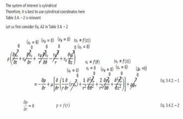
The pressure across the cross-section at a particular length in laminar flow through a pipe does not depend on the radial position This is an important insight
