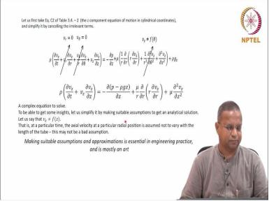
So, if this is the case, then we can take equation C2 it is still laminar flow. So, we can take C2 still flow in layers, so we can take C2 and C2 gives you this z component of equation in the cylindrical coordinates and that is this equation. If it cancel out the terms the first term which we were canceling, pretty much till now cannot be canceled because we said the velocity in z direction is the z direction let us same varies with time.
