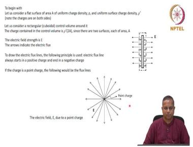
To begin with, let us consider a flat surface area A. Here this is a flat surface. I have just drawn a section of it therefore, it looks like a rectangle. It has another dimension into the screen here. Flat surface of area A of uniform charge density  $\rho$  connect charge density is  $\rho$  and uniform surface charge density as  $\rho$ ' surface charge density is density per unit mass density per unit area, in this case, surface charge density therefore  $\rho$ ' is density per unit area.
