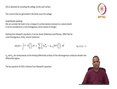
And the basis for design of EEG is the Maxwell's equations. EEG is obtained by recording the voltage on the skull surface you can have all those leads that go out and measure the currents that are generated in the brain caused the voltage which are measured. And simplistically speaking, again, very simplistically speaking, we can consider the brain to be a charge of a certain density enclosed in a volume which is the skull.
