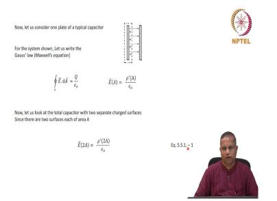
Now, we are going to consider one plate of a typical capacitor which is this. The capacitor has 2 plates. So, there are positive charges on one side of the plate along here in this capacitor for the system shown let us write the Gauss' law which is Maxwell's equation.
