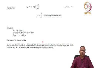
For water  $k_e$  happens to be about 0.01 Siemens per centimetre. Recall the units of conductivity Siemens per centimetre  $\epsilon$  is about 80 times the permittivity of free space for water this you may recall from your working out of problems from your high school pre engineering levels therefore, and you know that  $\epsilon_0$  is  $8.85*10^{-12}$  Farad per centimetres therefore, its 80 times that.
