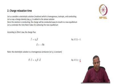
The second is a totally different concept is called charge relaxation time. Let us spend some time on this. Let us consider an electrolytic solution which could be a medium which is homogeneous properties are the same; well mixed isotropic it does not change with direction and conducting. So, this is our electrolytic solution the medium which is homogeneous isotropic and conducting.
