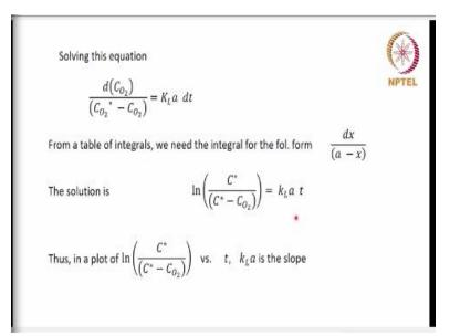
If you solve this equation, right, this is a differential equation right. If you solve this equation with an initial condition right you get d C<sub>02</sub>. This is a long term here recall, d C<sub>02</sub> in concentrations one side they have 1 by C<sub>02</sub> \* - C<sub>02</sub>, this C<sub>02</sub>. So, the long term arises because of this and this straightforward K<sub>L</sub>a dt, so t terms comes here. So, d [(C<sub>02</sub>)/(C<sub>02</sub>\* - C<sub>02</sub>)] = K<sub>L</sub>a dt.
