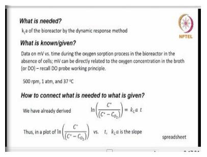
So, we look at what is needed first in this case,  $K_La$  of the bioreactor by the dynamic response method, what is known or given. We have data on millivolt versus time during the oxygen sorption process in the bioreactor in the absence of cells, millivolt can be directly related to oxygen concentration in the broth of DO.
