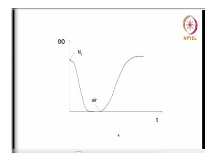
The way it is done is as follows, we plot, we look at, we measured that and we measure that plot dissolved oxygen in the broth versus time. And the experiment we do is as follows, we first purge the liquid with nitrogen to physically strip out all the oxygen that is present in the broth, ok. So, you pump it with nitrogen, that nitrogen replaces the oxygen on the broth, therefore the oxygen concentration in the broth drops gradually till it is zero.
