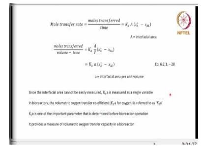
Welcome back, we are looking at a trans coefficient approach, we are taking this specific example of oxygen transfer in bioreactors, oxygen supplied to bioreactors. After a lot of discussion we have come up with this formulation, the moles transferred for you know volume per time is a certain  $K_xa$  times  $X_A^* - X_{AL}$ ,  $X_A^*$  is the liquid side concentration of oxygen which is an equilibrium with the bulk gas side concentration.
