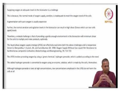
Supplying oxygen at adequate levels to the bioreactor is always a challenge ok, the bacterial or the aerobic microorganisms gobble up oxygen ok. And to supply at adequate rates is always a challenge, this is because a normal mode of oxygen supply which is aeration is inadequate to meet the oxygen need of the cells ok, that is the reason here. And augmentation with pure oxygen is usually expensive you cannot use oxygen cylinder, oxygen cylinders are expensive.
