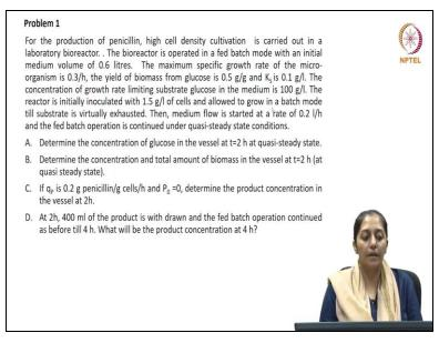
So we will try to do some practice with these problems. If you see on the slide the problem states that for the production of penicillin high density cultivation is carried out in a laboratory bioreactor. The bioreactor is operated in a fat batch mode with an initial medium volume of 0.6 liters. The maximum specific growth rate of the microorganism is 0.3 hour inverse the yield coefficient of biomass with respect to the substrate which is glucose here is given as 0.5 gram per gram.
