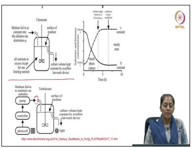
So, this is a simple schematic of a chemostat and turbidostat. So as I said earlier if you see the chemostat given on the top here the volume will remain constant shown by the dotted line. It is not changing and here in a turbidostat there is a controller which controls the flow rate of the pump and the calibration of the pump. And there is an optical sensing device which will continuously monitor inside the reactor or the broth.
