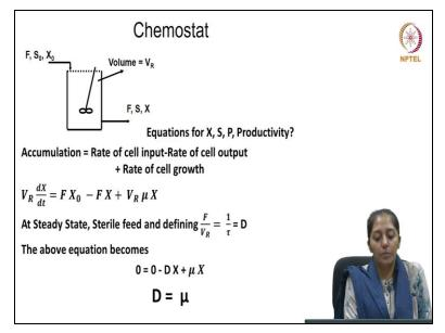
If you do a mass balance across this ideal chemostat for the biomass and reply, so if you do a mass balance, which means if we apply the content equation the rate of accumulation of the Biomass will be equal to the rate at which the cell is coming inside the reactor minus the rate at which the cell mass is going outside the reactor plus the rate of cell growth. Obviously we are assuming an obviously there is no under all practical conditions. There is no consumption of biomass taking place.
