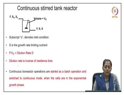
So let us note down some of the notations which will be used when will be designing continuous stirred tank reactor. If you can see the schematic on the screen that is an inlet stream showing F are the volumetric flow rate of the field. S 0 as the field substrate concentration and X 0 as the Biomass concentration present in the feed coming inside the reactor. The volume of the reactor is V R.
