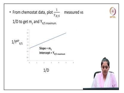
So you can see the plot your apparent yield coefficient which you measure as a function of the residence time. So as residence time increases which means the dilution rate decreases the y apparent yield coefficient also decreases. So this is the plot which has been made here. So 1 by Y AP is y and in terms of 1 by D as x so your intercept is your 1 by Y x by s theoretical and your slope is m s which is K d by Y x by s which is equal to your maintenance coefficient.
