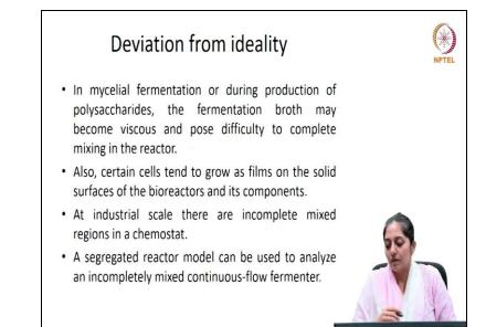
Now let us see a deviation from ideality. Like for example in mycelial fermentations now in mycelial fermentations or during production of polysaccharides for example the fermentation broth may become viscous and therefore pose difficulty to complete mixing in the reactor. Sometimes certain cells they tend to grow as films on the solid surface of the reactors and its component. At industrial scale there are incomplete mixed regions in a chemostat. So then in
