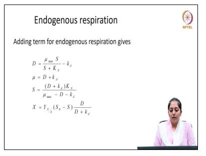
So let us see if there is endogenous respiration then how do we take into account that term in a continuous reactor. So in a continuous system we know that at steady state D is equals to mu where mu in case of endogenous respiration will be the net specific growth rate and when there is endogenous respiration it will be actual specific growth rate minus K d. We have done already earlier where K d is the rate constant for endogenous respiration.
