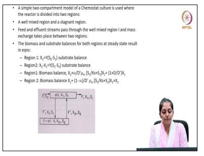
So there is a well known model which is called as two compartment model a simple model for a chemo start culture which can be used in such a scenario. Where the reactor is divided into two regions. A well-mixed region and a stagnant region. So if you see the schematic shown on the slide the field and the effluent streams they pass through the well-mixed region which has been given a subscript one.
