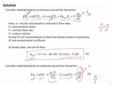
So now in order to determine this let us first list down what has been given to us and do a mass balance across this reactor. So, if you see the dotted line it is your system boundary and we will do a mass balance across the system boundary for the biomass. So, if we do the material balance, then FX 0 is the rate at which the biomass is coming inside the reactor. So, if you have noticed in the schematic F is the flow rate of the feed inside the reactor.
