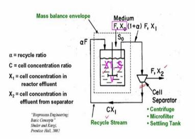
If you see the schematic which has been provided on the slide and the various notations where alpha stands for the recycle ratio, capital C stands for cell concentration ratio in the recycle stream versus the stream which is coming out of the reactor. X 1 is the cell concentration in the reactor effluent which means the stream which is leaving the reactor and X 2 is the cell concentration in the effluent from the separator.
