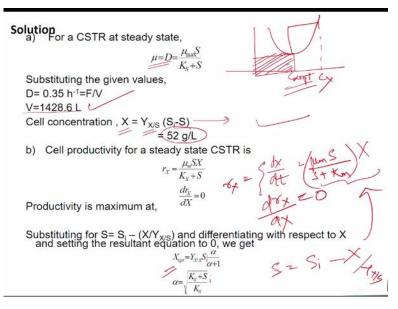
So now let us do the first part. So, if you are using a CSTR and there is a single CSTR being used, so then at steady state specific growth rate is equals to dilution rate. The culture is following Monod's model. Let us see what is given to us. Flow rate has been given. So now once the flow rate is given and we have been given the value of S inside the reactor coming outside the reactor which is 5 grams per liter.
