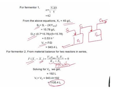
Once alpha is known, we can find the value of X for the maximum productivity. We determine the value of residual substrate concentration using the biomass. So now if you notice this S 1 is the stream which is coming out from the first reactor and if two reactors are in series. So, we have come to know the optimum biomass for the reactor in the first reactor.
