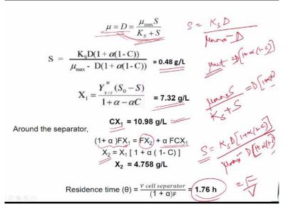
Then assuming that the specific growth rate of the culture is following Monod's model. So if you remember for a chemostat without cell recycle mu was equal to mu max S upon K s + S which is equal to D in case of steady state. And then finally the rearrangement would lead to an expression to determine S in terms of the dilution rate which used to be K s D upon mu max – D.
