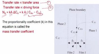
So, as I said earlier we will assume two-film theory to explain the mass transfer in the gasliquid interface. So, to generalize the rate of mass transfer we know is directly proportional to the driving force for the transfer and in this case the driving force is the concentration difference. So, it is directly proportional to the driving force and also to the area which is available for the transfer to happen.
