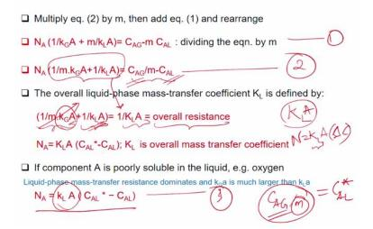
So, if you multiply equation 2 here which explains the rate of mass transfer of component A through the liquid boundary layer. So, if we multiply this by m, so m into C ALi we know can be replaced as C AGi and so m into C Ali. So we will multiply this entire equation by m and if we then add after multiplication the equation 1 and this is now can be written as N A. Then and if we bring all the constants together and the variables on one side, we end up in this equation.
