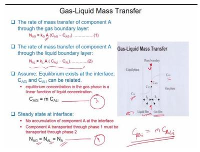
So, now let us derive some expressions to explain the gas-liquid mass transfer. So, the rate of mass transfer of component A, so if you see this schematic here, let us see the diagram where A is your entity which is transferring from the gas phase to the liquid phase. So, C AG stands for the concentration of that component A in the gas phase, bulk of the gas phase. Then as it crosses the boundary layer, the gas film, so there are two fictitious films across the interface.
