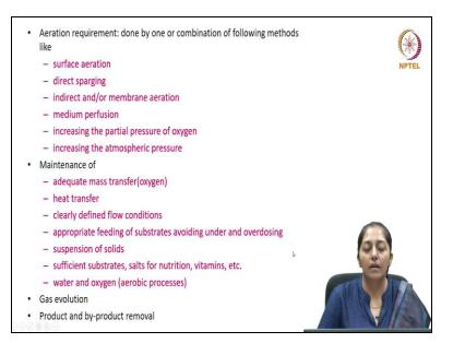
Further there are different ways in a bioreactors by which we can supply aeration to the organism like for example in some of the bioreactor designs aerations is done through the headspace which is called as surface aeration that can be direct passing. This is the most frequently used method of providing oxygen to the organisms, which is direct sparging inside the bulk medium or indirect sparging using membrane aerations this is generally used for Share sensitive cultures.
