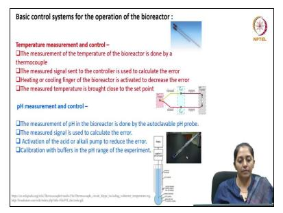
And talking about the control systems present inside the reactor for temperature control and measurement generally we have temperature probe. This probe is based on the principle of a Thermocouple so what happens that the temperature of the reactor is measured buy this probe and the measured signal is sent to the bio controller, which is used to calculate the error. Now this error is the difference between the measured temperatures of the liquid broth inside the reactor versus the set point.
