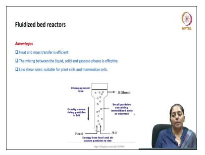
Nw immobilized cell bioreactors are further modified to overcome certain limitations of mixing in these reactors they are modified for better mixing by making them as fluidized bed bioreactors. The advantage is that there are better heat and mass transfer maintenance the mixing between the liquid solid and the gaseous phase is more effective and there are low shear rates in comparison to flee cell bioreactors.
