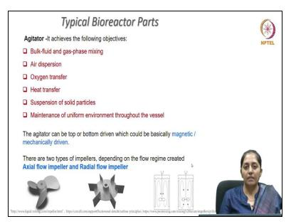
And talking about agitator it achieves objectives of bulk liquid and gas mixing provides dispersion of air, provides oxygen transfer from the gas bubble to the liquid broth. It facilitates heat transfer throughout the liquid broth and also from the liquid brought to the external coolant which is circulating to maintain the temperature of the reactor. Then it also helps in suspension of the cells aur solid particles inside the reactors during the cultivation does not allow them to settle.
