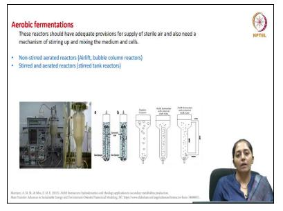
Talking about aerobic fermentation: In aerobic fermentation the different types of reactors. They can be classed as non stirred aerated reactors stirred aerated reactors. These reactors should have adequate provisions for supply of sterile air and also need a mechanism for starting up and mixing of the medium and cells. So under non stirred aerated reactor some of the examples are like airlift reactors or bubble column reactor.
