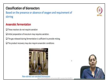
Give brief Idea on these different classifications basically the presence of oxygen or the absence of oxygen requirements, the fermentations can be classed as aerobic or anaerobic. In anaerobic fermentation the reactor they do not need large aerations initial preparation of inoculum all the might require little aeration. But the production does not need aerations. And the gas, which is released during the fermentation is sufficient enough to create adequate fixing.
