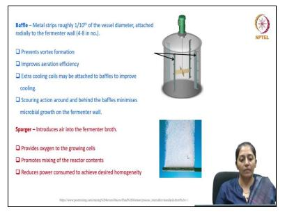
Baffles as I said earlier, baffles these are nothing but metal strip stainless steel strips roughly 110th of the vessel diameter attach radially to the fermenter walls. The function it helps in the vortex prevention of the vortex because if the vortex forms then it will lead to the appearance of dead zones at the corner of the reactors. So to avoid the dead zones which can hamper uniform mixing and uniform environment inside the reactor baffles are placed.
