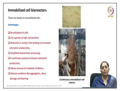
Then another type of reactors are called as immobilized cell bioreactors. You can see the pictures. These are alginate beads inside which the cell suspension has been encapsulated. So immobilize bioreactors they generally used to enable Re utilisation of cells till the viability is intact one can run high cell density cultivations. It enables reduction in the contact time leading to higher volumetric productivity.
