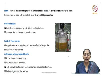
Talking about the anti foam: Now foam is formed due to entrapment of air as my seals which are made of the proteinaceous material from the medium or due to the cell lysis which have detergent like properties. That mostly happens in plant cell fomentation or animal fermentations where sometimes the medium components required proteins or amino acids or hormones or when the cell lysis happens and proteinaceous material components come out from the life cell into the broth.
