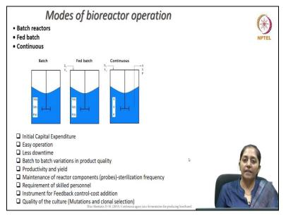
Even in a given reactor configuration thare can be different ways of cultivation. So there are basically three different ways cultivations are carried out. One is a Batch Mode of cultivation, then fed Batch Mode and the other is continuous mode. So these are three basic ways for modes of cultivation in bioreactors. Now batch reactor as you can see on the left most side of the slide. It is a closed system.
