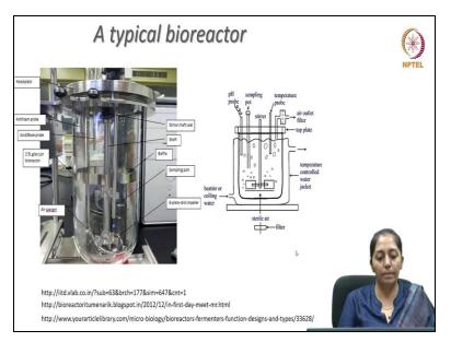
As you can see on the slide this is a schematic for a typical bioreactor with its different parts, which we discussed earlier. So there is a head plate frequency on the top then inside the glass vessel at the centre you will see the shaft which has impeller attached to it the photograph pictures soon has Sixth place disturb in impeller, which is mostly used for microbial fermentation. Then you will see a half u-shaped rod just ending beneath the impeller the bottommost impeller.
