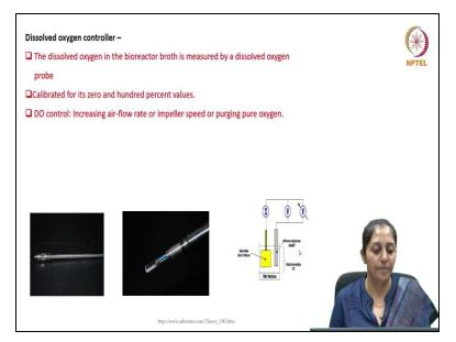
Then talking about the dissolved oxygen probe: The dissolved oxygen in the reactor broth is measured by dissolved oxygen probe it is based on the principle of Galvanic or polarographic electrodes. The schematics hear the schematically shows a polarographic electrode where the membrane at the bottom. It is selectively permeable to oxygen and the oxygen get reduced at the noble metal electrode due to which the current flows and it is measured as proportional to the oxygen tension of the broth.
