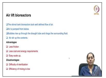
Most frequently used reactor design. Involves stirred tank reactor configurations, but depending on certain requirements airlift reactors have been introduced. Like for example the stirred tank bioreactor still AC well-defined flow of air the air is pumped from below and the bubbles as they arise up through the draught tube it drags the surrounding fluid and on the way it stirrups the contents.
