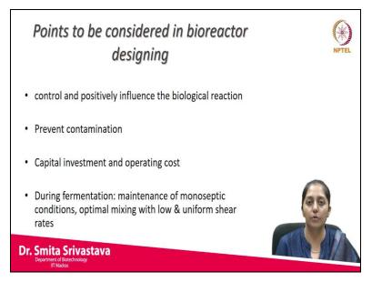
Welcome back students. So in the last class we stopped at the discussion on points which have to be considered when we are designing bioreactors. So, just to go through it once more time I am when we are designing bioreactors one should ensure that the bioreactor design should be able to control and positively influence the biological reaction. Further the bioreactor design should be able to prevent contamination.
