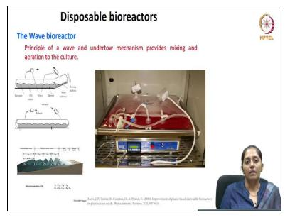
There are new set of reactor designs which are now been commercially utilised which come under disposable bioreactor classification where the reactor body is use and throw types. The mixing it is majorly meant for fermentation which do not require large amount of mixing or aeration where the specific oxygen demands are low like in case of animal cell fermentation and plant cell fomentation.
