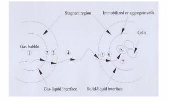
Steps for oxygen transport from gas bubble to cell
