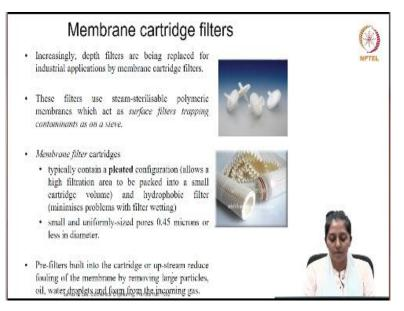
So, increasingly depth filters are being replaced for industrial applications by membrane cartridge filters. These filters, they are steam-sterilisable polymeric membranes, which act as surface filters, trapping the contaminants as on a sieve. So, membrane filter cartridges, they typically contain a pleated configuration as shown in the picture here, which will allow of high filtration area to be packed into a small cartridge volume.
