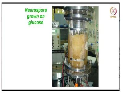
If you see the picture here, it is a filamentous fungi and neurospora, which has grown on glucose. You can see how much volume growth. It is all growing adheres to the stainless steel parts of the reactors, you can see the film adhere to the baffles, nothing is visible.
