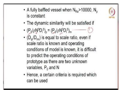
Like for example, for a fully baffled vessel. We can assume that N Re would be greater than 10 to the power of 4, which means it will be in the turbulence region and your power number can be constant. Let us take an example of rustling turbine. So, it can be 10 constant at a value of 6. So, then the dynamic similarity will be satisfied, if the power numbers are same at the prototype and the model type.
