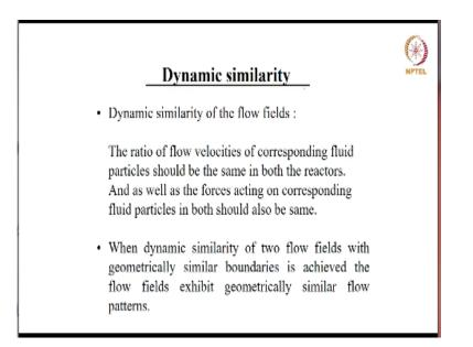
And what does dynamic similarity means? Dynamic similarity is with respect to the flow fields. It means that the ratio of the flow velocities of the corresponding fluid particles should be the same in both the reactors. And as well as the forces acting on the corresponding fluid particles in both should also be same. So, when dynamic similarity of the 2-fold fields with geometrically similar boundaries is achieved, the flow fields exhibit geometrically similar flow patterns.
