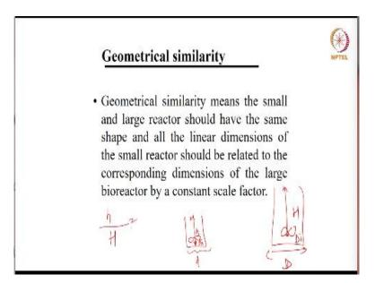
Now, to understand, what is geometrical similarity? Geometrical similarity means, the small and the large reactor should have the same shape and all the linear dimensions of the small reactor should be related to the corresponding dimensions of the large bioreactor by a constant scale factor. Suppose, we have 2 reactors, here, the diameter is small d, the height of the tank is small h, here the diameter is capital D and the height of the tank is capital H.
