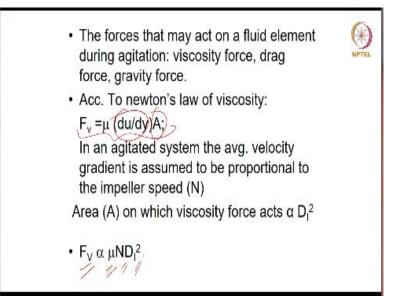
So, the forces that may act on a fluid element during agitation, they include viscous force, drag force, gravity force. Now, according to Newton's law of viscosity, we know viscous force can be given in terms of the stress strain relationship. Now, in an agitated system, the average velocity gradient, this which we have written as du by dy, this can be assumed to be proportional to the impeller speed.
