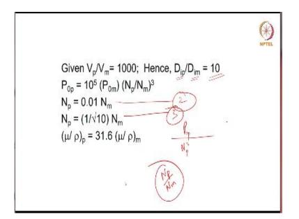
So, let us see. Now, we know that the ratio of the volume or the prototype to model type is given 1000. So, from here, we can find the ratio of the diameter of the impellers of the prototype and the model type which will be your 10. Let us go one by one. Let us take the first requirement, the N Re to be same. So, if N Re is equal at the 2 levels, the correlation between N and D i, because the liquid properties will not change at the 2 levels.
