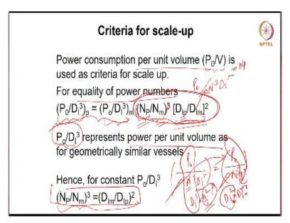
So, let us take these scale-up criteria one by one and try to derive relationships between the different operating parameters are the 2 scales. So, power consumption per unit volume is the first scale-up criteria. If you do equality of power numbers and do the rearrangement, and then your D i to the power of 5, if it can be broken up as D i cube and D i square separately. So, we know that power number is P 0 by N cube D i the power of 5. Is not it? And you have density.
