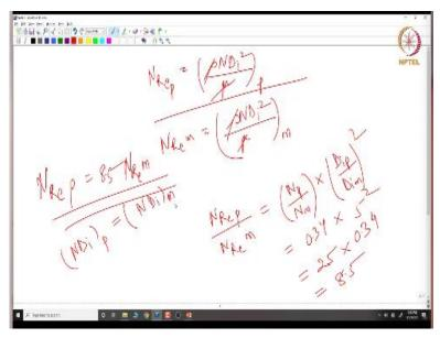
So, N Re is what? Rho ND i square by mu. So, let us call this for prototype and N Re for model type is rho ND i square by mu for the model type. Now, mu and rho are the same. Now, in terms of the prototype, if we divide this, so, N Re at prototype to N Re at model type will become equal to N p by N m multiplied by the D ip by D im the whole square. N p by nm, if you notice N p by N m how are they related for constant P 0 by V was this. N p by N m is equal to 0.34.
