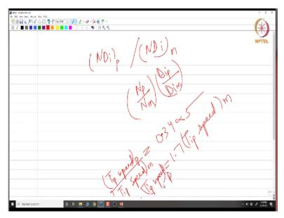
So, tip speed at the prototype by tip speed at the model type, if you do, then we know that N p by N m is 0.34 and D ip by D im is 5. This is the ratio of the tip speed at the prototype and the impeller tip speed at the model type. So, if you need to find the relationship between them, this comes out to be 1.7 times tip speed at the model type will be your impeller tip speed at the prototype. This is what has been shown here in equation 3 and equation 2.
