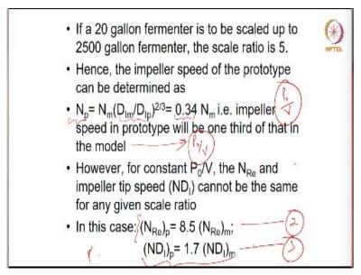
Let us take an example. If a 20 gallon fermenter is to be scaled-up to 2500 gallon fermenter then we know the scale ratio would be 5. The impeller speed of the prototype then can be determined, if P by V is the scale-up criteria. Then in that case, we know now, the diameter ratios can be given as 1 by 5. So, therefore, your impeller speed at the prototype will become 0.34 times of the impeller speed at the model type to keep your power per unit volume constant other 2 levels.
