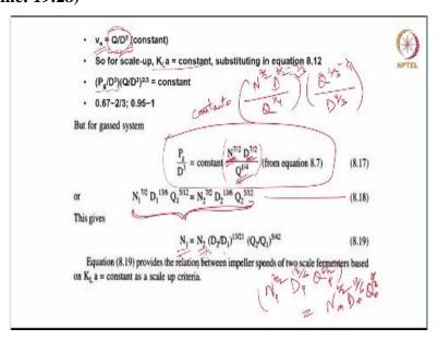
Now, the superficial gas velocity can in turn be written as in the form of the volumetric gas flow rate and the diameter of the impeller square with some constant. So, now again the superficial gas velocity can be written in terms of Q and D as Q by D square. Now, for scale-up, we know that K L a is constant. Now, for making K L a constant, now, this P g by D cube
