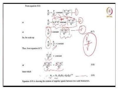
So, if the gas power requirement per unit volume is the scale-up criteria, which means P g. So, the gas power requirement is being called as P g, the un-gas power requirement is P 0 or P here shown on the slide. So, it is said that power per unit volume will be the scale-up criteria and from the previous equation which we called as 1, we can relate the gas power requirement with the un-gas power requirement.
