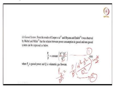
So, if we have a gas system, so, right now, the power per unit volume, the P 0 was the ungassed power requirement. So, if we have a gas system, will there be a variation in the correlation between the impeller speed and the diameter ratio? So, there is an empirical relationship between the power consumption in gassed and non gas system which is shown here by equation.
