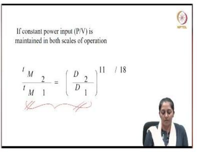
So, if apart from the constant mixing factor, if we can imply constant power input per unit volume at both the scales, then further your correlation 3 can be reduced to only correlation relating the mixing time with the diameters.
