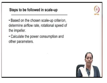
Based on the chosen scale-up criteria, determine the airflow rate, the rotational speed of the impeller at the large scale of the prototype. And calculate the power consumption and other parameters.
