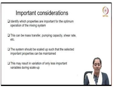
So, what are the important considerations? First, we need to identify which properties are important for the optimum operation of the mixing system. Now, this can be mass transfer or
