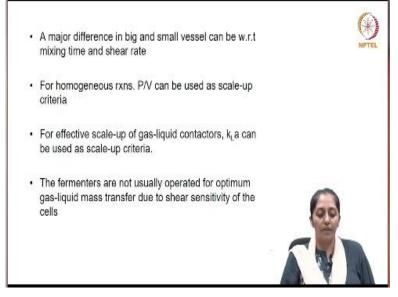
So, the major difference in the big and the small vessel can be with respect to the mixing time and the shear rates. Now, for homogeneous reactions, power per unit volume can be used as a scale-up criteria, cells are uniformly suspended, it can be called as a homogeneous mixture. For effective scale-up of gas-liquid contactors, where 2 phase interactions are important gasliquid interactions then K L a can be used as a scale-up criteria.
