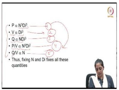
So, effectively, this is how power input is related to impeller speed and diameter of the impeller. This is how volume of the tank is related to the diameter of the impeller. Knowing the diameter of the impeller is proportional to the diameter of the tank, some scale ratio. And the volumetric gas flow rate is also related to the impeller speed and the diameter of the impeller, power per unit volume can also be related now.
