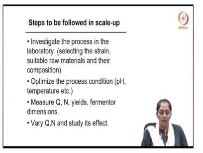
So, what are the basic steps which one must follow during scale-up? First, investigate the process in the laboratory, select the strain, the suitable raw materials and their composition. Optimise the process conditions like pH, temperature, etcetera. Measure the properties like volumetric gas flow rate, the impeller speed, various yield, parameters, yield of biomass with respect to substrate, yield of oxygen biomass with respect to oxygen consumed, yield of product with respect to biomass.
