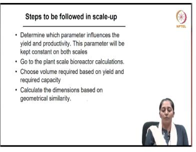
Now, determine which parameter influences the yield and productivity most. This parameter should then be kept constant on both scales. Now, going to the plant scale reactor calculations, choose the volume required based on the yield and required capacity, calculate the dimensions based on geometrical similarity.
