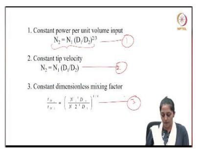
So, let us see the correlation. Once again for constant power per unit volume, the correlation between the impeller speeds and the diameters is shown here. Then for constant tip velocity which was N D i, this will be the correlation which is very simple. Then constant dimensionless mixing factor will give as the correlation here. If you remember, equation 1 shown here was a correlation for dimensionless mixing factor.
