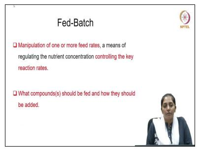
So what are the different permutations and combinations which can come out as a feeding strategy. While designing a feeding strategy in a fed batch this may involve which substrate are to be fed at what concentrations they are to be fed. How long they are to be fed inside the reactor and at what fashion they are to be fed which means at what flow rates whether constant flow rate or increasing flow rate so that is also to be determined.
