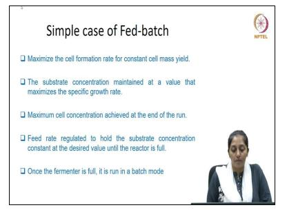
Let us take a simple case of fed batch and try to design the fed batch kinetics. Now the objective of running a fed batch operation is to maximize the cell formation rate for constant cell mass yield. So constant cell mass yield is your yx by s maximizing cell mass concentration is your x. The substrate concentration maintained at a value that maximizes the specific growth rate.
