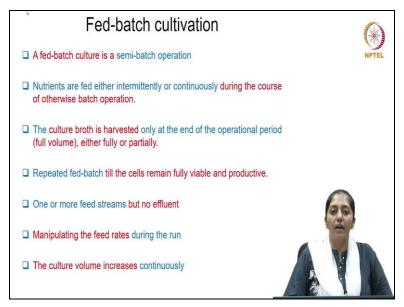
Welcome back students, so in the last class we were discussing design of batch reactors. Now in this class we are going to move ahead with the design of fed batch reactors. So if you remember in the introductory lectures I spoke about the different types of and modes of cultivations in which batch mode of cultivation was one which we call as batch reactors. And then there was fed batch mode of cultivation.
