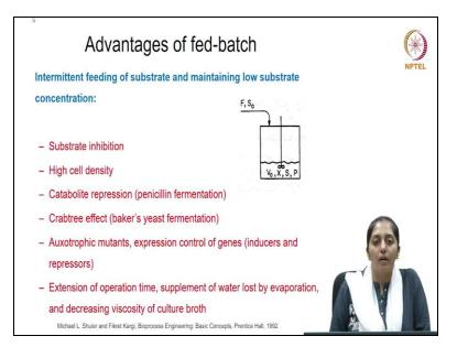
Now let us take some examples as advantage of a fed batch process. Intermittent feeding of substrate and maintaining low substrate concentration, now let us take some examples like substrate inhibition. Now imagine when inside a reactor there is only one feed stream or there is an inlet stream but there is no outlet stream then the substrate inhibition. If you remember the earlier classes in batch operation what was substrate inhibition?
