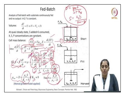
So now after discussing some of the advantages of fed batch process, let us see now how to design a simple fed batch process. Now here we will assume that in this fed batch process if you can see the schematic on the slide. We will make certain assumptions. We will assume that this fed batch process is a constant feed flow rate process which means there is a flow rate f of the inlet feed going inside the reactor and it is constant.
