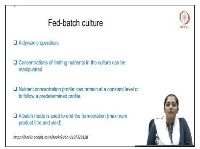
So because the inlet feed is continuously coming inside the reactor the volume is changing the concentrations of the variables therefore will be changing. So it is a dynamic system. Concentrations of the limiting nutrient in the culture therefore can be manipulated. Now the feeding can be controlled in a manner such that the nutrient concentration inside the reactor can be controlled at desired levels.
