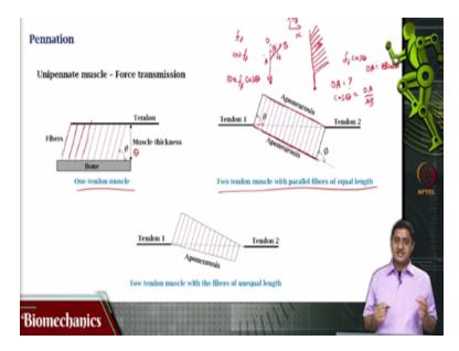
So, let us look at this with the bit more detail. The fibres are attaching like this, in the case of the unipennate case. The fibres are all parallel to each other and they are attaching like this the angle of attachment is sum theta, is the angle at which the fibres are attaching. There are many cases many possibilities in which this can happen. One is there is only a single tendon muscle, the fibres are all attaching to the bone directly like this.
