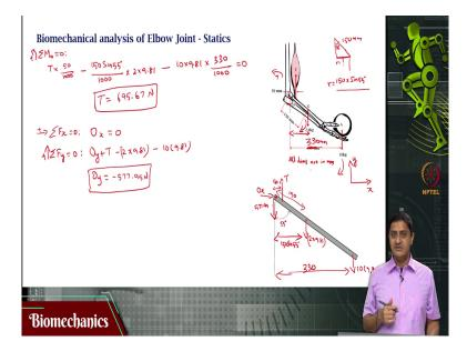
This is a rough free body diagram of the situation. So, the forearm free board diagram is given this angle is given to be 55 degrees um this is the joint O and a known muscle tension T is acting here I do not know the value of this force but what I do know is that this distance is 50 mm all the dimensions are in mm when I am drawing all the dimensions are in mm. This is 50 mm what I also know is at a distance of 150 mm along the forearm not in the XY axis.
