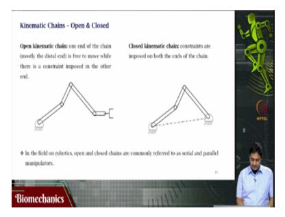
Then you have open kinematic change and closed kinematic change. For example, I can consider the arm system as an open kinematic chain. The end effector is open it is not attached to any particular point or a body or another body. So, one end of the chain mostly the distal end. So, this is in this case this is approximal and that is the distal end. Or mostly the distal end is free to move it can move anywhere, not anywhere it can move it is free to move.
