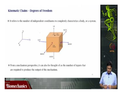
We have discussed this in some of the previous videos, what is degrees of freedom? The number of independent coordinates that are required to completely describe a given body. So, I have this body, I have this object. This object, can translate upward or downward accelerate upward or downward one degree of freedom, can accelerate to the left or the right or can translate towards you or towards me.
