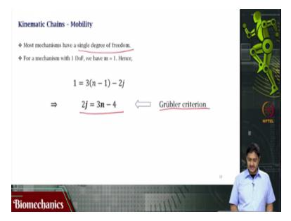
Now for a mechanism with one degree of freedom that means it has mobility m = 1 I substitute m = 1. Many mechanisms that are under discussion will have only a single degree of freedom and our analysis will also have a single degree of freedom whether it is. Once you substitute m = 1 immediately the number of joints and the number of links are related to each other and 2j = 3n - 4.
