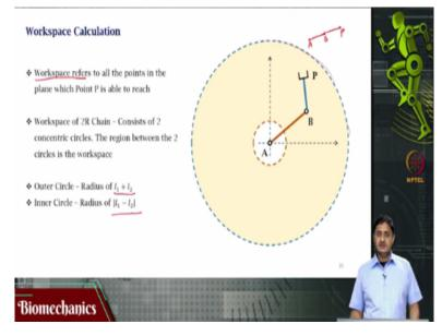
We are interested in computing workspace. What is this workspace? It refers to the set of all points in the plane within to which this point P will be able to reach. For example, in two link chain in a 2R chain it consists of two concentric circles the region between the two circles is the workspace. So, I have one concentric circle which is one of these two concentric circles which is the outermost circle.
