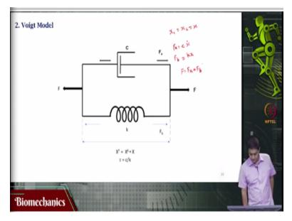
This is the Voigt model; this is a dashpot in parallel with the spring. In the Maxwell model what we had was a dashpot in series with the spring. Here you have a in parallel with the spring which means that there will be qualitative difference in the response of this model when compared with the Maxwell model. That makes sense but we do not know what exactly that is, in other words we have not yet done the mathematical formulation of this which we will do.
