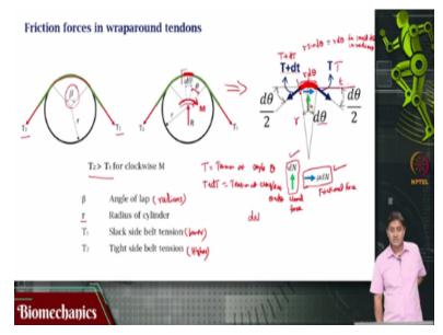
Now that situation can be modelled similar to a cylinder that on which a belt has been wrapped around or wound around. Let us say that the rope has contact with this cylinder for an angle beta in radians and this rope or this belt has two tensions T 1 and T 2. If there is an external rotation that is applied as shown in this picture an external rotation capital M that is applied, T 2 can be assumed to be greater than T 1 for the sake of discussion.
