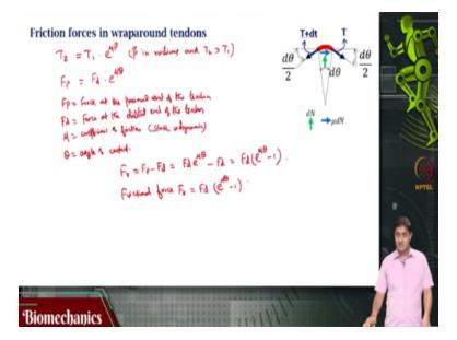
The Euler Eytelwein formula is T 2 T 1 e power mu beta where beta in radians and T 2 is greater than T 1 this is the Euler Eytelwein formula. In biomechanics this is usually written as the force on the proximal side of the tendon is the force on the distal part of the tendon times e power mu theta, where theta is the angle of contact, mu is the coefficient of friction F d is the force at the distal end of the tendon.
