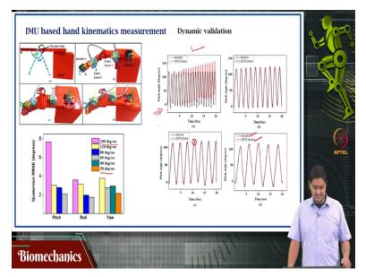
To perform the dynamic validation, we made again with 3D printed another system that could house, these PCB's this (()) (18:28) PCB's and our electromagnetic tracking sensors that are from polymers. These are polymers liberty electromagnetic tracking sensors, of course these are sensitive to metals around them and it gives us a different principle. Remember we discussed how this works in one of the previous videos.
