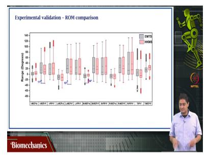
We also compared just for safety purpose just for as a check as a post check. We also compared whether the range of joint angles that you get in a set of all movements performed by a set of all participants are comparable between the electromagnetic system and our IMU-based system and we found that they are almost comparable. There were some differences in some cases and those differences are all highlighted here.
