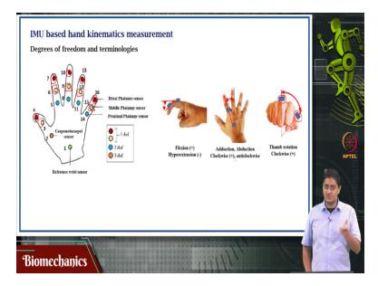
Here we discuss how we can use similar principles to measure full hand kinematics. How many different sensors would you need and how many degrees of freedom would your model have. So, remember the distal phalange only fluxes and extends, the middle phalange also the same. So, essentially the dip joint or the distal interferential joint and the pip joint or the proximal interferential joint are modelled as hinge joints or one degree of freedom joints.
