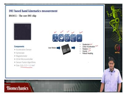
So, this is all fine, what is the particular method that we use? We use the Bosch BNO055 IMU chip and we built our own board. So, in our lab we have developed our own board around this Bosch BNO055 chip and developed the instrumentation around this chip this is not an advertisement or an endorsement of Bosch BNO055. You can use any IMU you want and any microcontroller you want.
