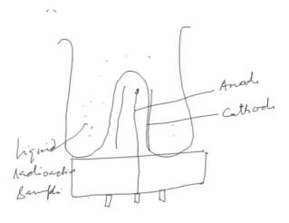
Now, this could be used for different kinds of samples, but there is one annular well type counter, which is utilized for the liquid samples, which could be utilized for liquid samples and it could look something this sort, which is, you have same similar sort of thing, but it is like you have a place for so there will be a cathode which is metalized cathode surface. Then, there will be anode here, which is anode wire in the center, the liquid sample will be filled in here.
