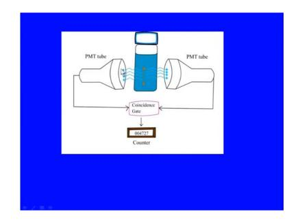
This figure shows, how to photo multiplier tubes have been put in here, you can see there is one photo multiplier tube here, another here and the sample is in between. So, when signal reaches to both, then only it will be counted otherwise, it will not be counted. So, that is the one method to reduce the photo multiplier noise. There are other disadvantages also, one of the greatest disadvantage of scintillation counting is quenching.
