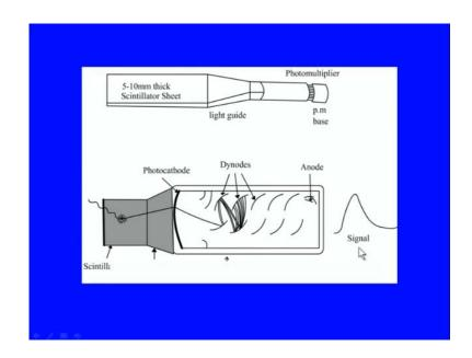
This is the photo multiplier tube, this we have explained earlier in case where, we were discussing stem electron microscope also. So, there is a scintillator which collects this light, these are converted to and through a light guide, they reaches to the tube, there is a photo cathode. These photons are converted to photo electrons, they are amplified and finally, signal is measured.
