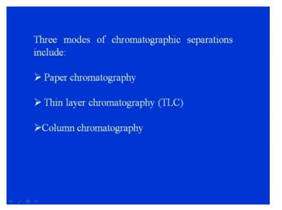
Now, there are three modes or rather we can say usually two modes of chromatographic separations. Now, here three modes where paper chromatography could be one mode it has been kind of replaced by thin layer chromatography. Paper chromatography and thin
