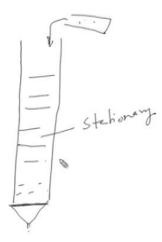
So, let me show you the how column looks like actually. Now, if you see the column the column is a simple tube like column structure which is closed on one side, it will be closed on both sides while running, but to support the matrix there is a filter a disc support with a filter the material will be filled with in this here, which is your matrix the
