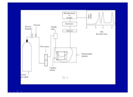
Now, here in this diagram, if you can see on your screen, it is a schematic of a gas chromatograph. It very nicely detects the different components of the gas chromatograph. Now, if you see from starting here, this is the carrier gas supply in a particular tank or cylinder. This carrier gas is supplied from here from this tank. As it goes through the tubing, there are pressure regulators and pressure meters.
