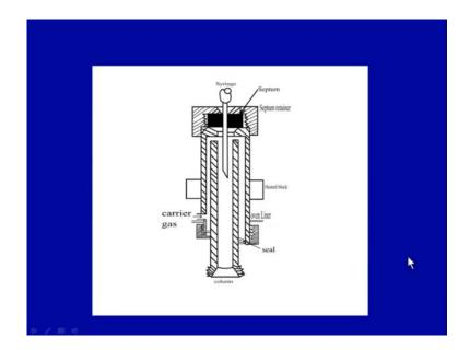
Now, this is a very typical representation of typical vaporiser, where you can inject the sample in here. As you can see on a screen, there is a syringe, which injects the sample in here through a rubber septum. There is a heat block and this is heated to very high temperature. So, the liquid could be converted to vapour instantly. Then once it is done, this will flush into the column, where it can be separated. So, this is the typical vaporiser, you can say a flesh vaporiser.
