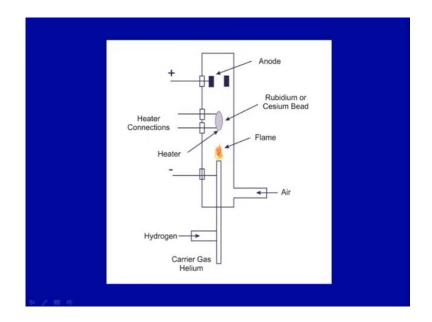
Another thing is here, there is a simple schematic like FID. Only detect here is a flame, which is a cooler flame. There are heater connections. There is a medium or caesium bead here and anode, which is collector here. As the comp analysts are ionised here than mostly nitrogen and phosphorous compounds, then the signal could be or could be recorded in here. Another detector, which is for particular kind of compounds is called electron capture detector.
