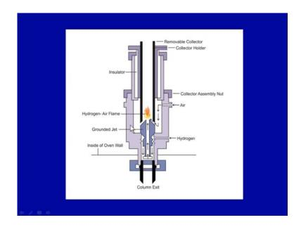
If you see the very simple schematic, here a flame ionisation detector, when you can see here, there is a flame here. There is a collector. You can say collector assembly wire. So, what happens is the exit or material is put in this flame. It ionises and the current is passed. The signal is recorded and destructible like grounded jet. There are a lot of hydrogen air flame is here. Hydrogen is supplied from here and air is supplied for the flame.
