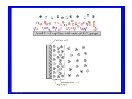
So, this figure kind of explains what I have already explained that there are fused silica capillary with negative charges. I said as I said at different ph, it will be charged differently. There is an external layer here which is shown here that which is like the cations compensating for negative charge on capillary wall. There is diffused layer which is here and as the applied voltage is applied, everything moves towards cathode. So, that is the phenomenon which is electro osmotic flow.
