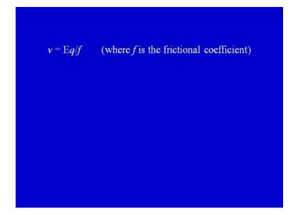
v equals E q upon frictional force or frictional coefficient, so that is the velocity a particular molecule will experience or will have when it moves through the, under the influence of electric field through a particular medium. Now, like I said, the more common term for the migration of charged particle is electrophoretic mobility.
