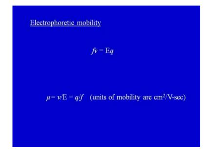
So, as the ion moves or accelerates, a frictional opposes the forward motion. So, in the beginning, the charged particle is put under the influence of the electric field, it will move towards the opposite electrode and it accelerates as it moves through medium. As it accelerates, the frictional force comes into existence and this frictional force will oppose the forward motion of the ion or the charged species.
