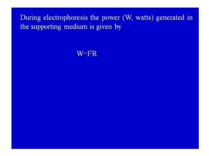
So, during electrophoresis, the power generated in the supporting medium will be given by this particular equation that is W I square R. The most of the power, which is generated here, is dissipated as heat. So, what is the problem here because of heat? Now, heating of electrophoretic medium or apparatus has lot of effects actually, several effects which are important here.
