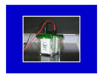
You have enclosed buffer chamber and these are the electrodes, two electrodes here. The gel apparatus is kept on here. As you switch on the electric current, this whole pattern will; the protein migration will take place and separation will take place. After the protein has been run, you can remove the gel plates from here. Gel plates could be separated and the gel could be put in the staining solution like say solution containing the Coomassie or any other dye and that could be visualized.
