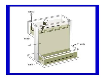
So, typically this is how it looks likes actually. If you see here, this particular one on the screen, this is tank buffer that is the top tank buffer and bottom tank buffer. So, this contains, this here contains the electrode buffer or you can call it running buffer. As this tip is showing here through pipette, you can load these samples in this wells very smoothly so that it diffuses out and settles down to the well.
