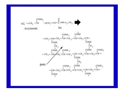
This figure here shows you, this is acryl amide molecule. What happens is that this is bis acryl amide and long chains of acryl amide are formed and like these two chains and in between, bis acryl amide gets inserted. As the cross linking occurs, depending on the concentrations, the pores will be created. So, polymerization of acryl amide is an example of free radical catalysis.
