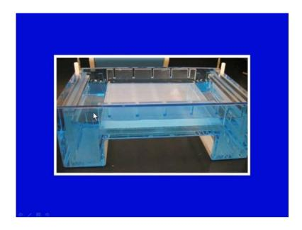
This is typical electrophoresis apparatus for horizontal, a typical horizontal gel electrophoresis apparatus for running the agarose gels. As you can see that here tank buffer is put and there will be two electrodes, which will be one positive and negative. The STS shape gel is placed and agarose gel is placed here. Then sample will be loaded and this we have discussed. So, the wells are created and the sample is loaded. The DNA will run towards the positive electrode.
