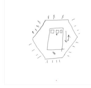
You have six legs in here. In field inversion pattern, what you have is gel loaded in here and you apply the electric field in two directions. One direction is in this direction and the other direction is in this direction that is at 180 degrees. So, accordingly these four electrodes, which are placed in here, will change. Either they will be negative or they will be positive. So, they will be either negative electrodes or positive electrodes accordingly.
