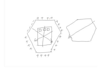
It is not perfect, but I think you can understand that. Now, you have like each leg contains this hexagonal array of electrode arrangement. Here, each leg contains 4 electrodes. I will just make one. These are 4 electrodes. These electrodes are made of platinum wires. So, what you can do is for now, the direction force on the DNA say there is a DNA molecule here.
